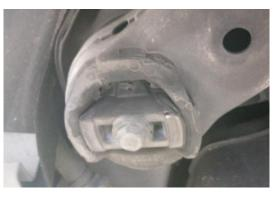
Figure 02 – Cradle Bolts to be loosened.
