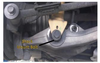
Figure 01 – Left Rear Lower Wishbone Control Arm
