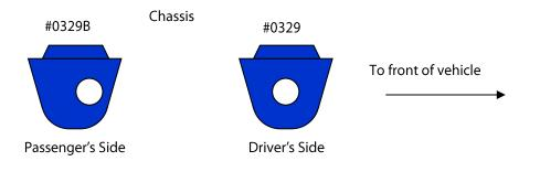
Kit # 0329BK – Passenger's Side & Driver's Side Increase Castor Settings Kit Install bushings as per diagram below
