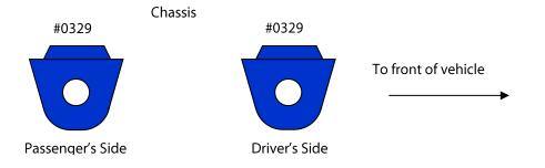
Kit # 0329AK – Passenger's Side Increase & Driver's Side Standard Castor Settings Kit Install bushings as per diagram below
