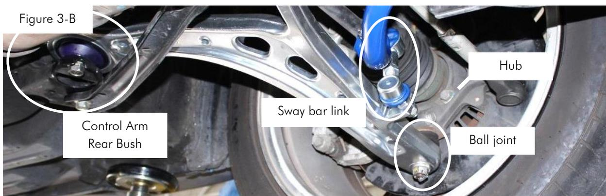
Figure 3 – View from underneath of the vehicle - Left Hand Side Control Arm installed
