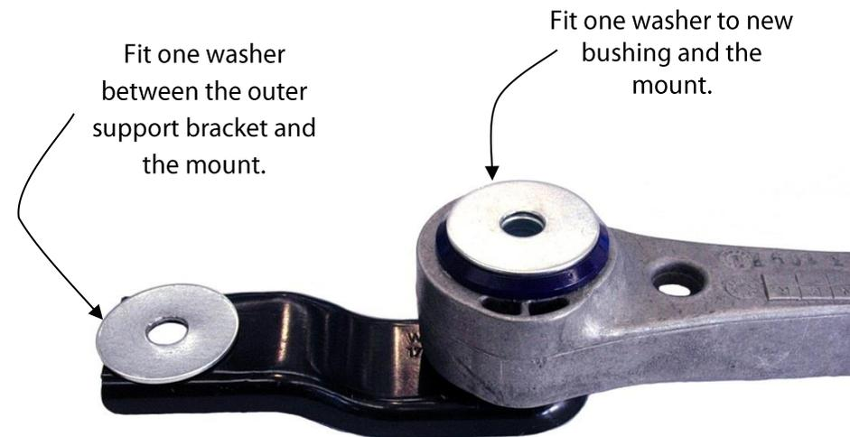
Offer the bracket to the vehicle as shown above.
