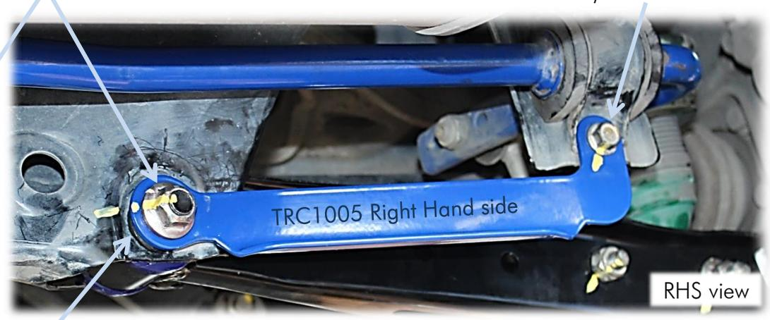
**Note** that the supplied 5mm washer should be placed between the brace and the sub-frame, as indicated in the pictures.
