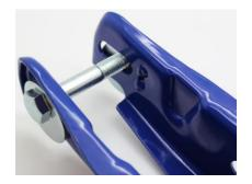
o Take the vehicle onto the wheel aligner and adjust the camber bolt to your desired result.
