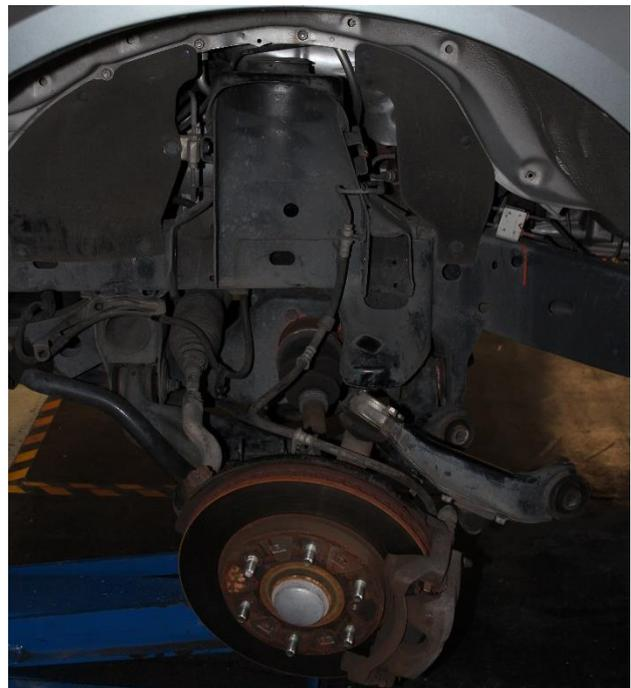
Picture 1: Front Strut Removal
