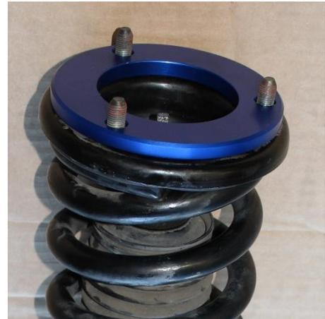
Picture 2: Strut Spacer on Strut
