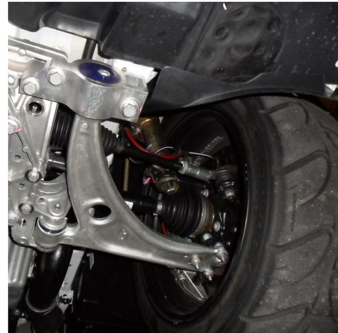
Figure 03 - View of underside of car right hand side shown with arm assembly installed
