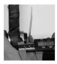
Because the tapered end of the crush tube extrudes away from the bush, while setting the bush offset position in the arm, please ensure that you measure from the end of the crush tube to the face of the housing (As shown in figure above).
