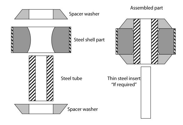
Note the orientation of the Spacer
