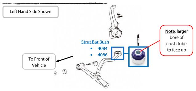
*Note:* Polyurethane bushings must be fitted to both sides of the vehicle.
