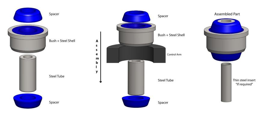
**Note:** In some applications a thin steel insert is used inside the original crush tube. This insert must be removed before attempting to remove the arm from the vehicle. During installation the insert should be re-installed into new steel tubes.
