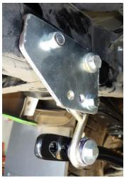
Note: Supplied is 2 different length links. The short ones are for STD height vehicles whilst the longer are for raised Vehicles to give more off-road articulation
