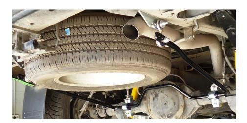
Recheck positioning making sure the bar is central and clear of all obstacles. Torque all bolts before lowering the vehicle off the stands
