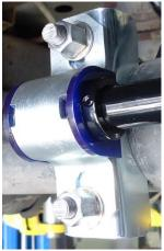
Note: the D/bush buts against the lock ring and in turn the U/bolt sits against the Brake hose brackets
