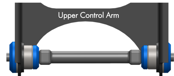
Bottom View of the bushes installed into the arm
