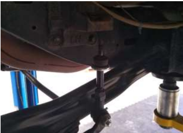
Fig 01 Sway bar link pin disconnected
