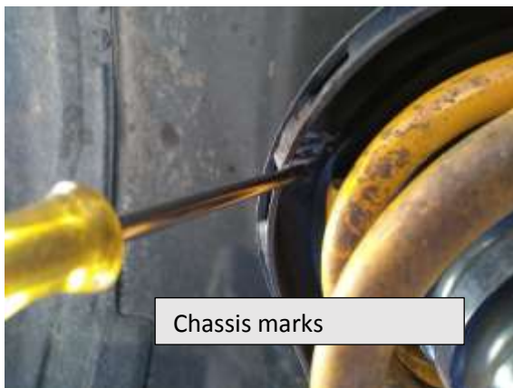
Figure 05- timing of the Spring and spacer (right hand shown)
