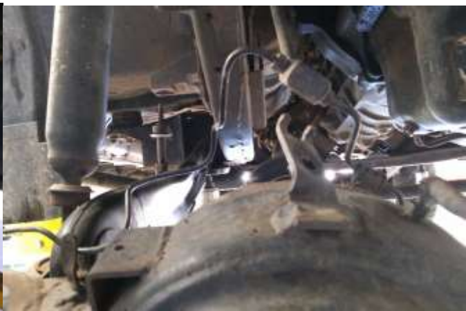
Fig 02 Brake lines and lower shock mount disconnected from diff
