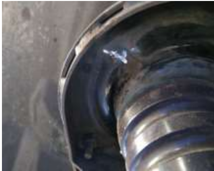
Fig 03 Marked spring seat showing step
