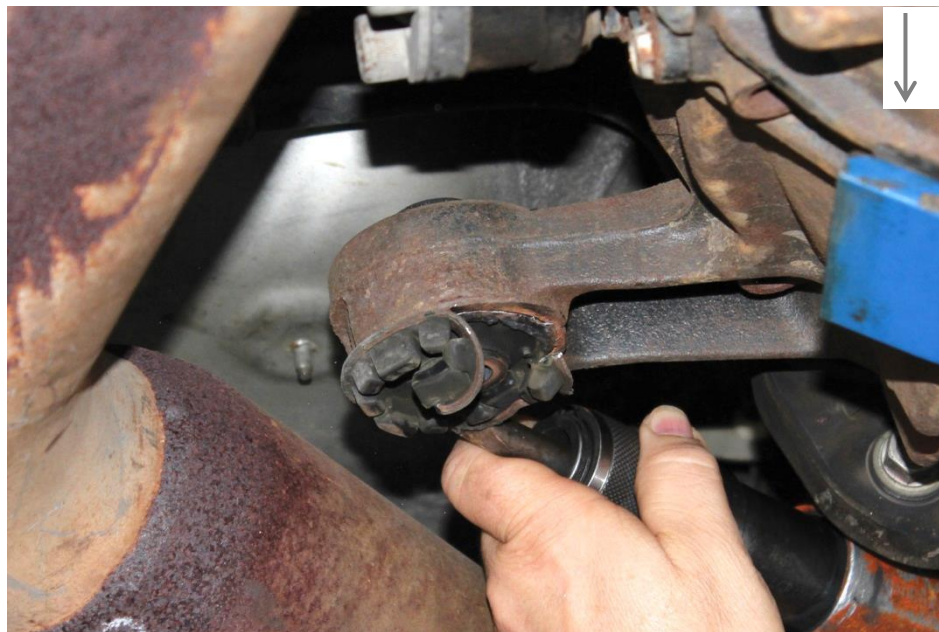
Figure 01 – Using an air chisel to cut the original bush flange.
