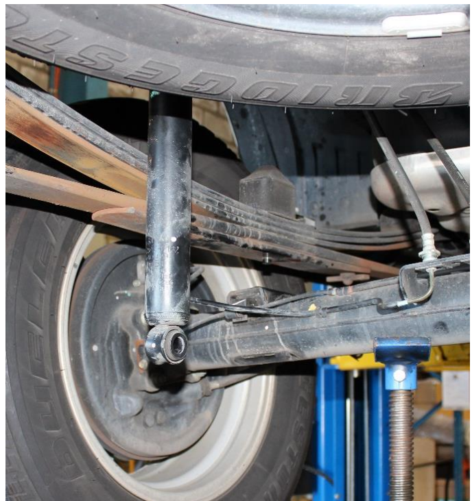
Picture 2: Installation of Raising Block
