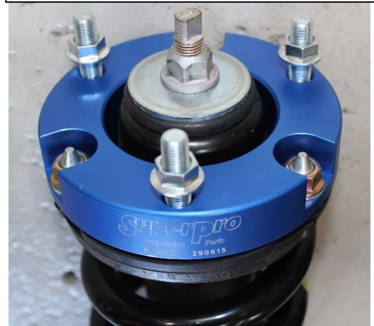
Picture 1: Picture of strut spacer on strut
