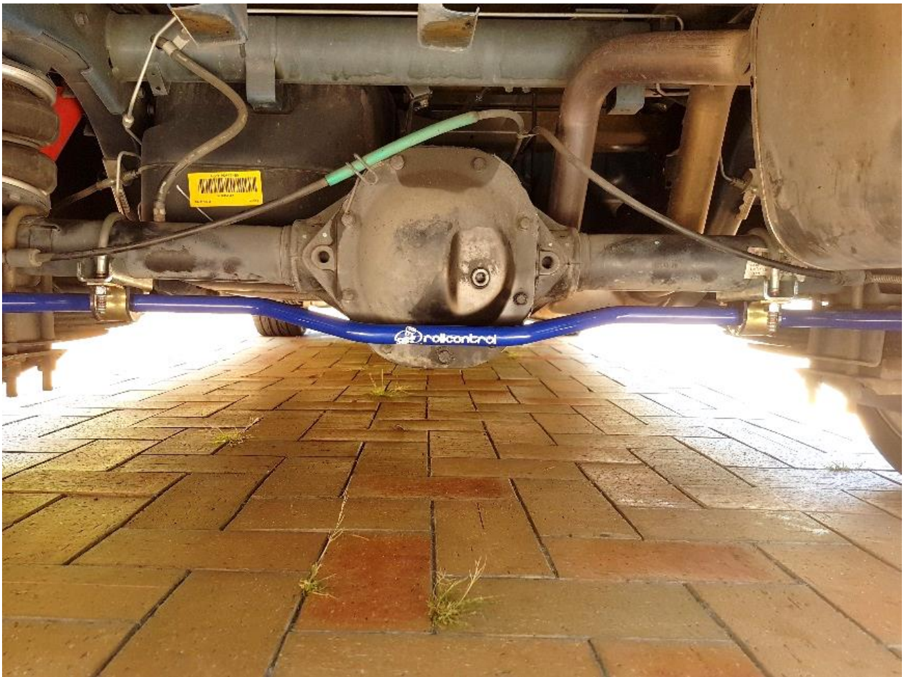
Figure 01 – Sway bar installation – Rear View.
