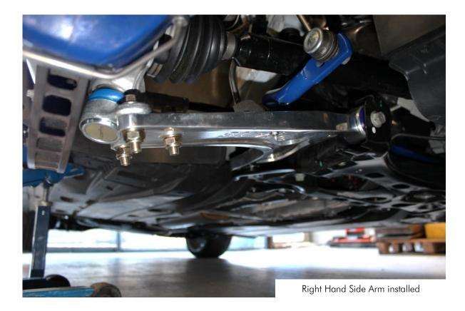
o Tighten all bolts to manufactures torque setting and carry out wheel alignment.
