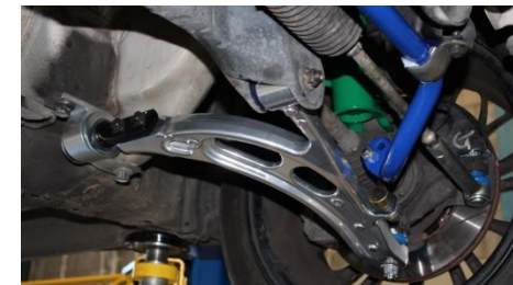
View of underside of car left hand side shown with arm assembly installed
