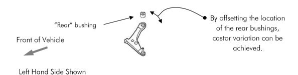
*Note:* Polyurethane bushes must be fitted to both sides of the vehicle.
