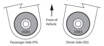
**Kit #2086K** – To counteract a slight pull to the left Single Offset – (passenger side caster increase & driver side no caster change)
