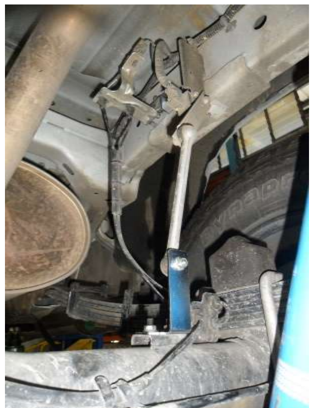
Completed assembly with new brackets installed
