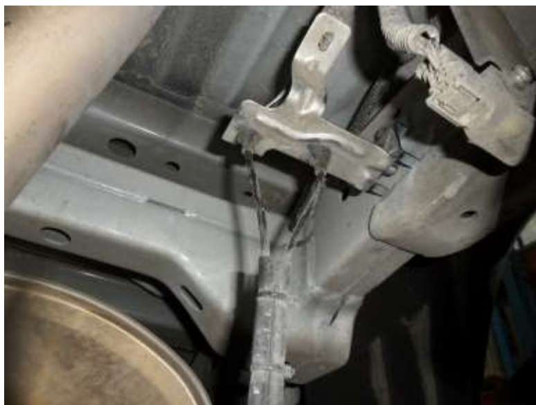
Re fixed bracket and ABS cables re attached
