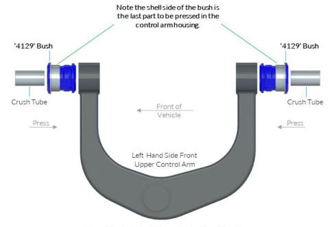
Figure 01 - LHS Front Upper Control Arm, Top View
