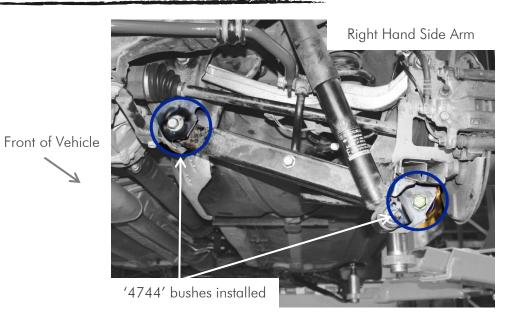
*Note*: Polyurethane bushings must be fitted to both sides of the vehicle.
