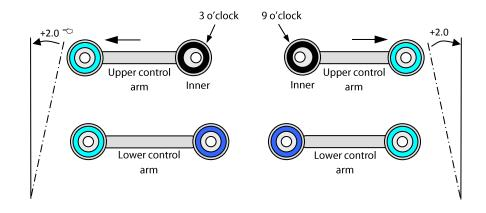
This diagram shows the maximum camber adjustment that can be achieved with this kit. Variation of this adjustment can be achieved by rotating the offset tubes in the bushings.
