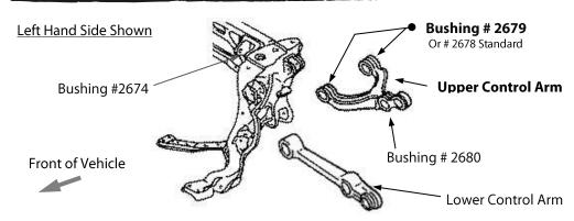
Note: Polyurethane bushes must be fitted to both sides of vehicle.
