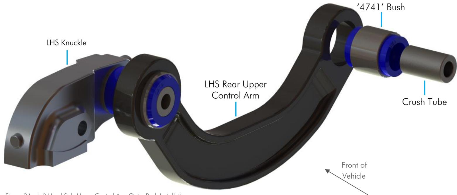
Figure 04 – Left Hand Side Upper Control Arm Outer Bush Installation
