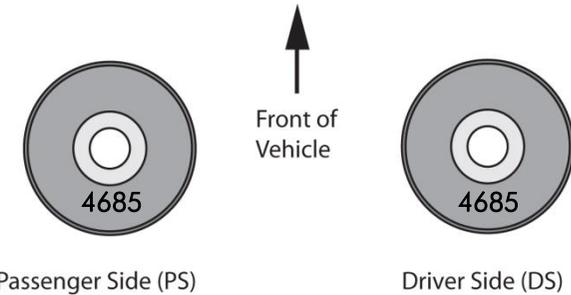
Kit #4686K – To counteract a slight pull to the left Single Offset, Passenger side caster increase (+0.5 degree).
