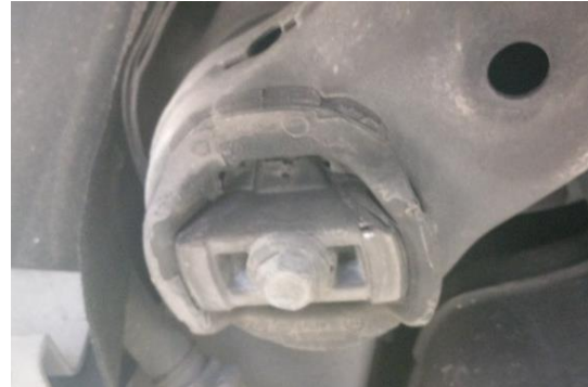
Figure 02 – Cradle Bolts to be loosened.
