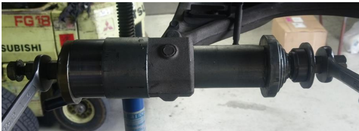
Figure 04 – Booker-Rod set up to remove pre-existing bushes.
