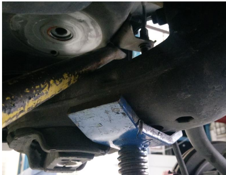
Figure 03 – Lowered Cradle being moved back for access to front bolt.
