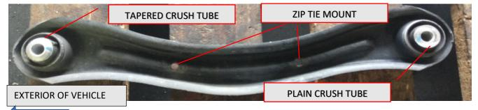
Figure 04– Left Rear Upper Control Arm displaying location of tapered crush tube.
