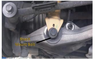
Figure 01-Left Rear Lower Wishbone Control Arm
