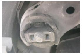
Figure 02 – Cradle Bolts to be loosened.
