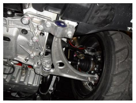
$\label{lem:continuous} \mbox{ View of underside of car right hand side shown with arm assembly installed }$
