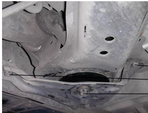
Figure 2: Bottom view of Cross-Member
