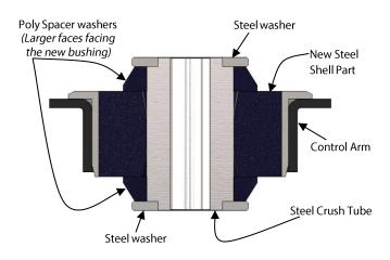
Note the orientation of the Poly Spacer Washers.
