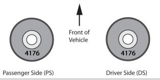
**Kit #5593K** – To counteract a slight pull to the left Single Offset, Passenger side caster increase (+0.5 degree).
