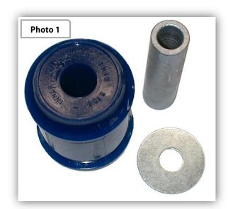
Remove radius arms from vehicle, and press out Original Equipment (OE) bushes from the radius arm to chassis position.
