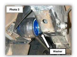
**Photo 3** – The washer must be used between the inner face of the bush and the spigot on the chassis rail. This ensures the arm does not drift sideways over the mounting spigot.
