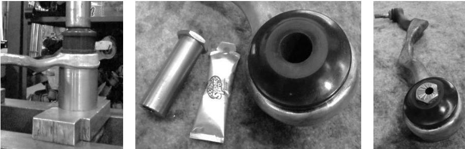
Figure 1: SuperPro Polyurethane Bushes and Crush Tube
