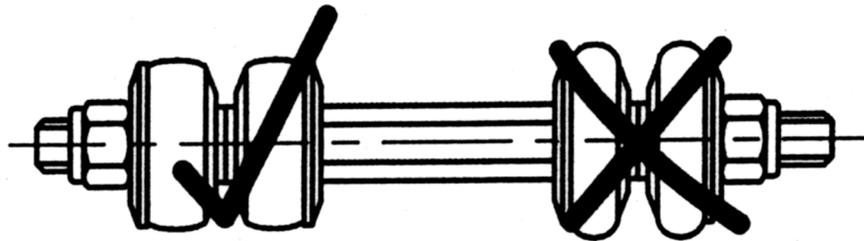
**Note:** Assemble washers as per drawing above (Cup towards bushing).
