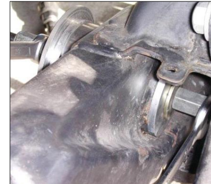
Figure 3 – Insertion of new outrigger bush
