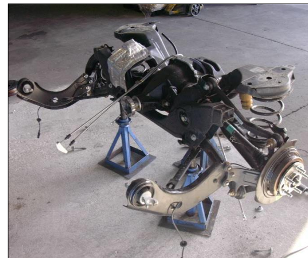
Figure 1 - Back end removed from vehicle
