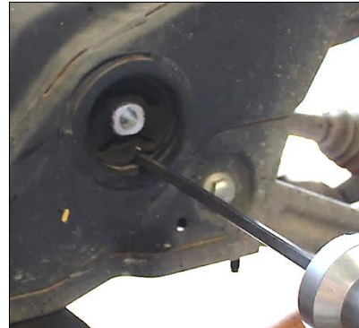
Figure 2 – Removal of differential outrigger bush
