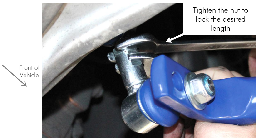
Figure 09 – Installing sway bar link on the left hand side
