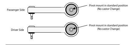
**Kit #3338K** - To counteract a slight pull to the passenger side Single Offset – (passenger side increase and driver side standard castor)
