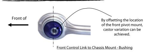
**Note:** Polyurethane bushes must be fitted to both sides of the vehicle.
