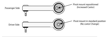
**Kit #2247K/#3339K** – To counteract a strong pull to the passenger's side Double Offset – (passenger side increase and driver side decrease castor)
