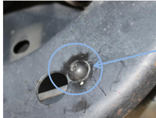
Figure 3 - Plastic clip holding ABS cable in place. Outside view
