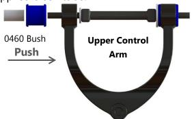
Arm assembly after new bushes are installed
