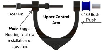
3) Re-use factory nuts and washers on the upper control arm and tighten to manufacturer's torque settings.
