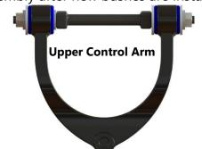
Refit the front upper control arms to the vehicle, tighten all fasteners to manufacturer's torque specification and carry out a wheel alignment
