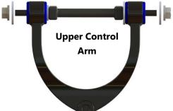
2) Next, Install 0460 bush into the arm followed by the supplied crush tube.
