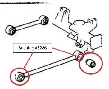
*Note:* Polyurethane bushes must be fitted to both sides of the vehicle.
