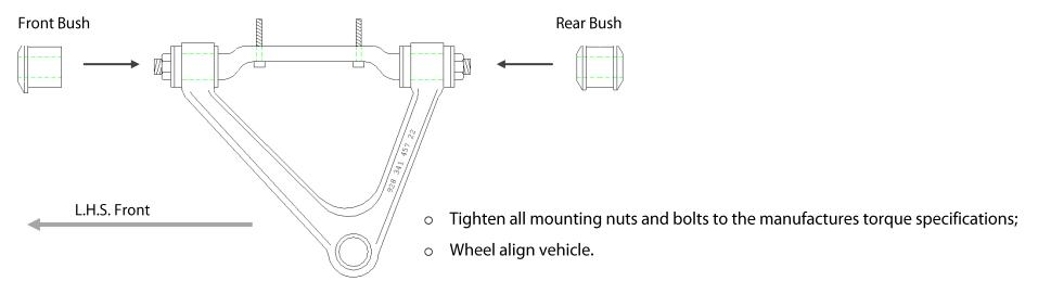
**Special note:** Upper control arm main retaining bolts must be tightened with the vehicle at ride height.
