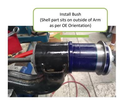
Note: Polyurethane bushes must be fitted to both sides of the vehicle.
