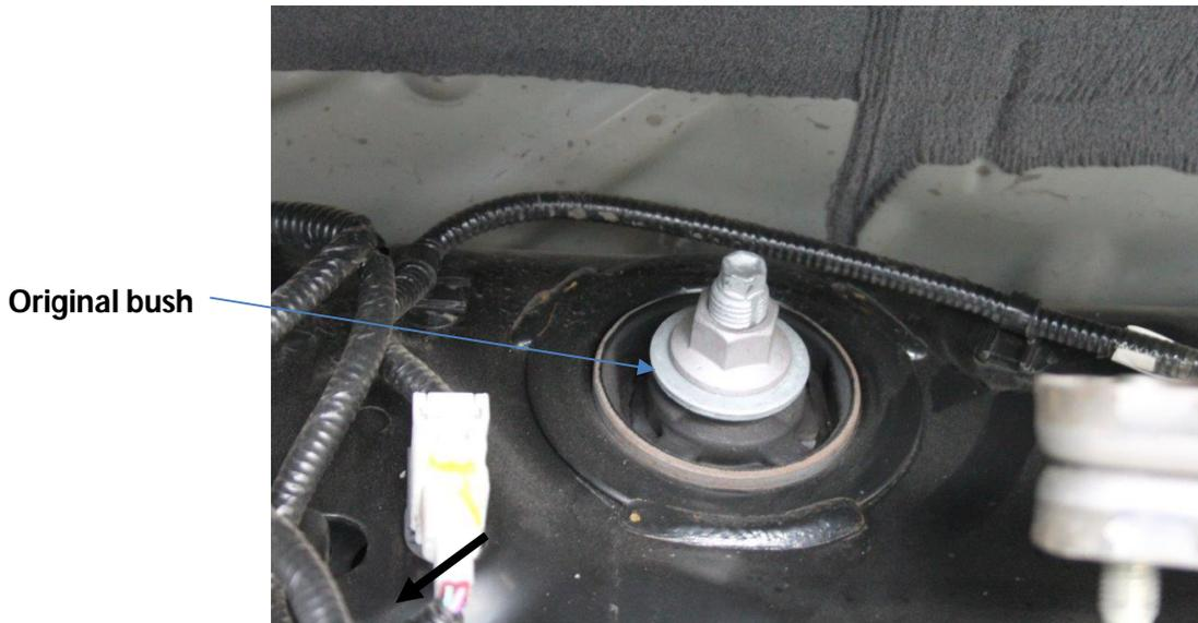
Note: **It is possible to remove and replace this bush without removing sub frame**
