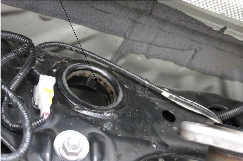
Note the outer shell of the bush should sit level with the cross member
