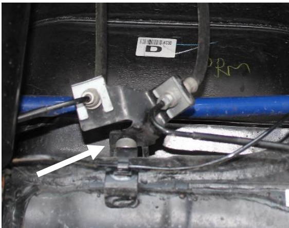
Picture 4: Rear lower brake hose mount spacer position
