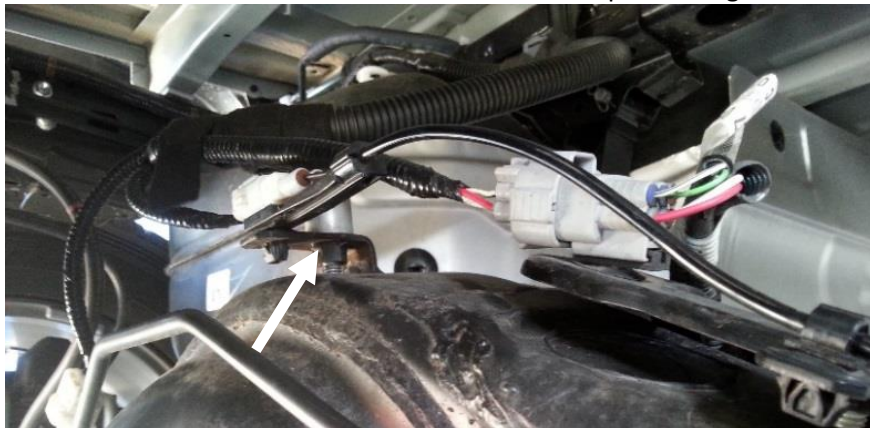
Picture 6: ABS cable mount position
