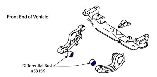
*Note:* Polyurethane bushes must be fitted to both sides of the vehicle.
