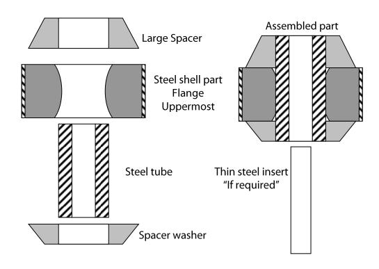
Note the orientation of the Spacer
