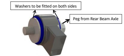
• Refit the rear panhard rod to the vehicle and ensure that all fasteners are torque to manufacturer's specification and carry out a wheel alignment.
