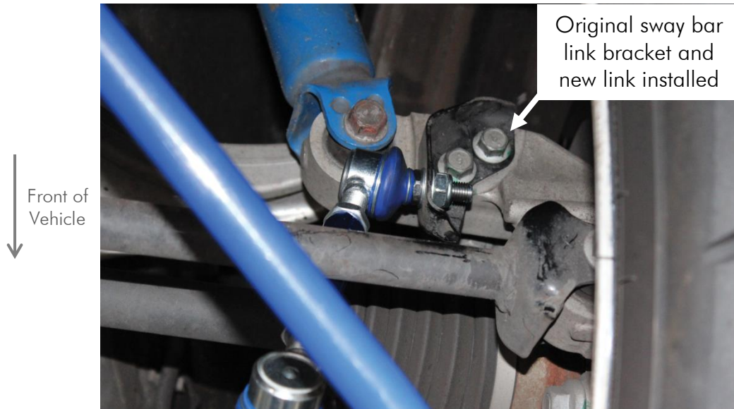
Figure 08 – New sway bar link installed on the original link bracket attached to the hub. Right hand side view
