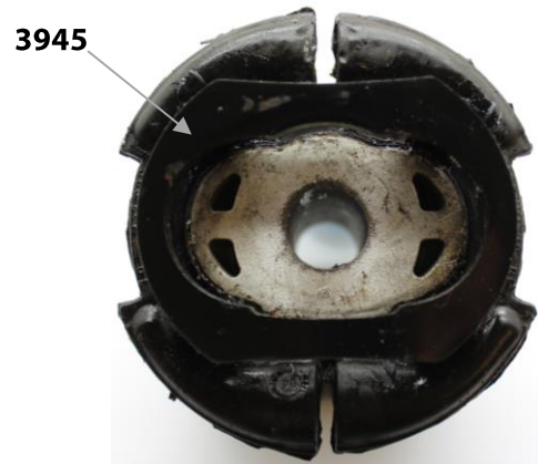
Rear lower subframe insert – note the shape of the polyurethane insert and match it up to the shape of the pin and push it in.
